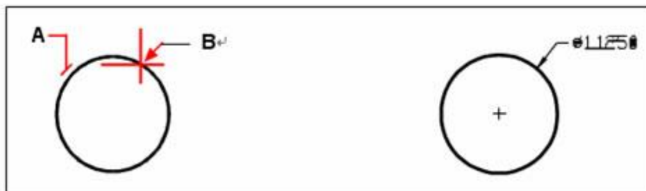
Select the circle (A), and then specify the dimension line location (B).
